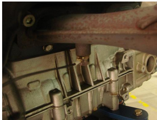
Figure 14 - Example of Temperature Sensor Installation Local
