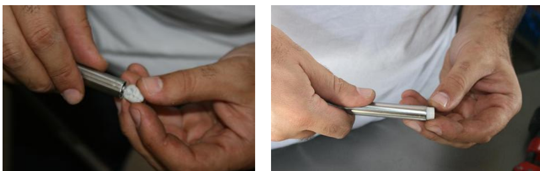
Figure 12- End Plug placement
