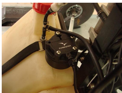
Figure 5 - Fuel Sensor Installation Example
