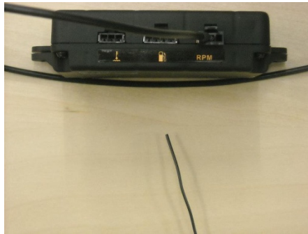
Figure 15 - RPM Sensor connection to M1
