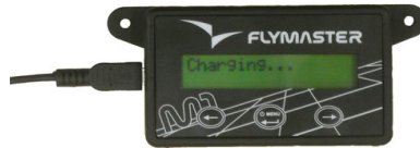
Figure 1- Battery charger connection
