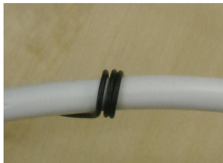
Figure 16 - Sensor Wraps Around Spark Plug Cable
